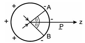
By considering elements of charge at A and B, say, where the surface charge density is the same (because of the symmetry of the problem) it is clear that there is only a z direction contribution to the E-field at the centre of the cavity - <u>all</u> of the charge on the surface of the cavity can be paired of in this way so there can be no non z direction contribution.
