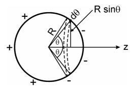
The surface polarisation charge density in this case is given by  $\sigma_{bound} = \underline{P} \cdot \hat{\underline{n}} = -P\cos\theta$  (the sign is due to the fact that  $\hat{\underline{n}}$  is an <u>inward</u> pointing unit vector).
