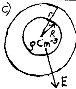
From the symmetry of the problem E is clearly directed in a radial direction. Considering a spherical surface of radius  $r > R$  we apply
