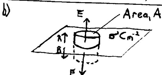
From the symmetry of the problem E is clearly perpendicular to the sheet.
