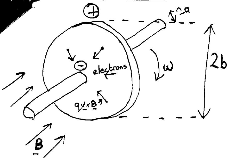
The  $qv \times \underline{B}$  Force on the electrons causes them to move in the direction shown (given the above  $\underline{B}$  and rotation directions) and hence there is an induced  $E$  field which eventually discourages further movement in a radial direction.
