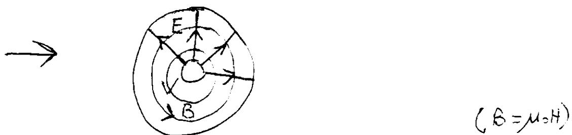
The Poynting vector  $S = \underline{E} \times \underline{H} = \frac{1}{\mu_0} \underline{E} \times \underline{B}$  gives the value of the power/area and is clearly always in the direction of  $\hat{r} \times \hat{\phi} = \hat{z}$ , along the cable, out of the sheet, in this case
