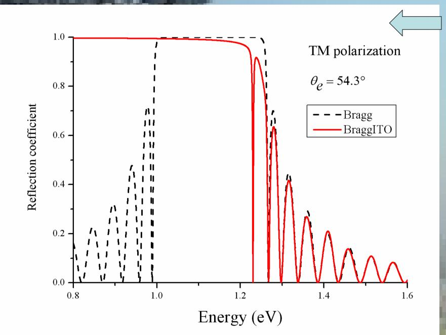
FIG. 2 TM polarization. The reflection coefficient as a function of energy at an external air/interface angle of 54.3°. Results for the air/Bragg reflector/glass substrate (Bragg) and air/ITO(1650 nm)/Bragg reflector/glass substrate (BraggITO) structures are shown. A distinct feature associated with an SPP at the ITO/Bragg reflector interface is present at 1.230 eV. A nominal collision term was employed in these calculations. The
